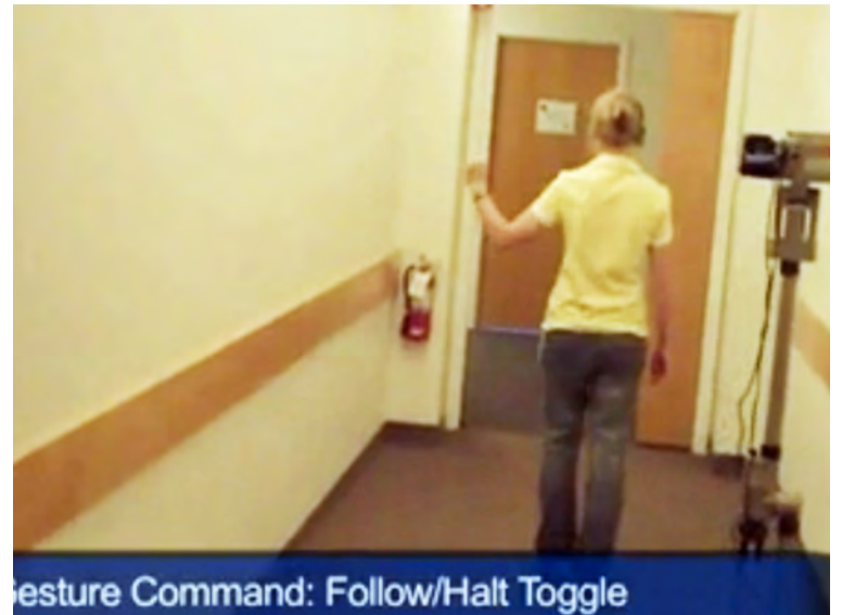
Hands-Free Robot Control using a special sign language and a 3D camera
